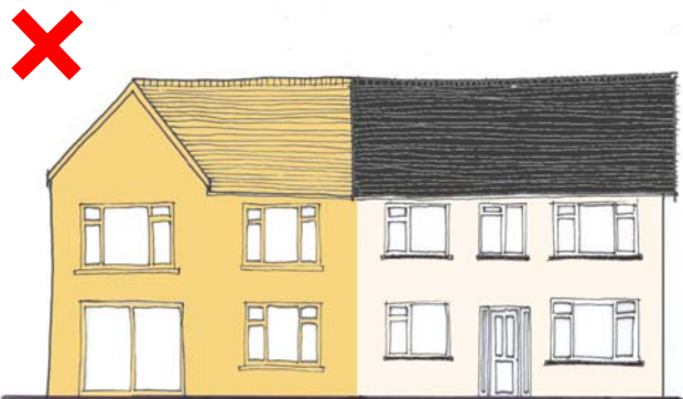
A poorly designed side extension that competes with the scale and form of the original house
