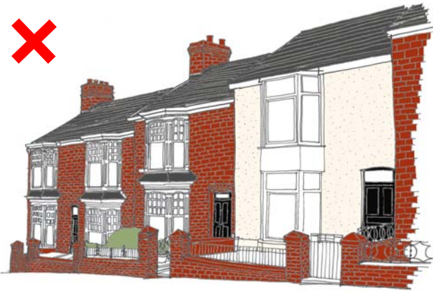
The use of inappropriate materials in this row of traditional terraces undermines the whole street
